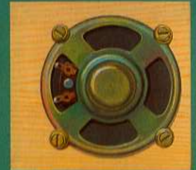
The Loudspeaker is mounted over the circle with 4 screws and cups
